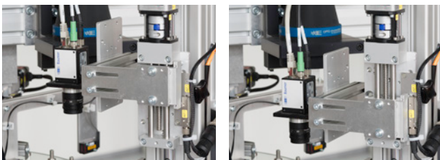
The positions of cameras and light fittings can be freely programmed within the traverse range of 45 mm.
